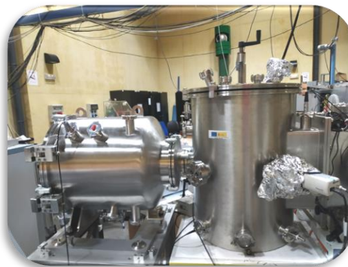
Fig. 3. Redesign of the vessel with a domed shape to avoid vacuum stress damage, and a 10 mm thickness PMMA port
