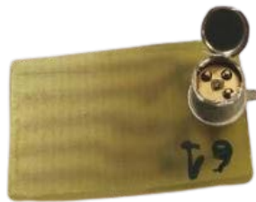
MOSFET 3N163 (Vishay) decapsulated
