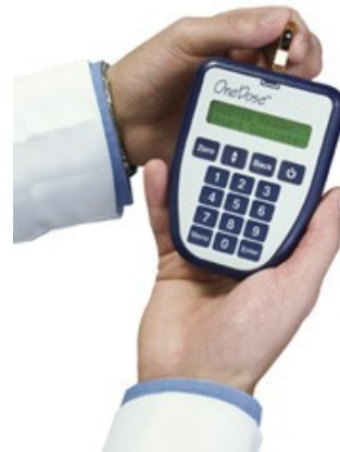
OneDose system: dosimeter patch and the reader
